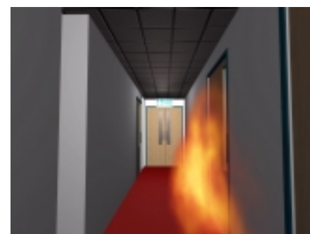
Figure 1: At the onset of fire, the emergency exit sign is fully visible.
